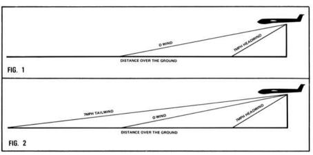
"fuselage angle" but with that same 7-mph wind now at your back (tailwind), a greater distance would be covered over the ground (see Fig. 2). The airspeed would still be 10 mph but the ground speed would now be 17 mph.
